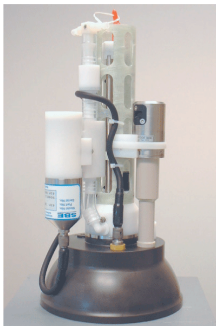
Figure 4: Photo of the top cap of a profiling float with the two most advanced oceanographic oxygen sensors installed side by side: The SeaBird Electronics Inc. SBE-43 electrochemical sensor is on the left, with the Aanderaa Optode sensor on the right. Field results from such dual-sensor floats are already available. (Photo from S. Riser)
